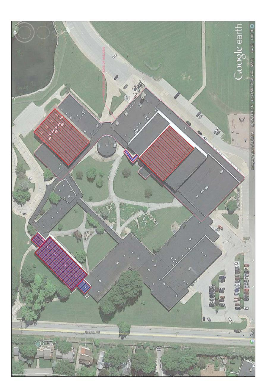
ASBESTOS CONTAINING TAR ROOFING (BOTTOM LAYER) - 9,120 SQUARE FEET
